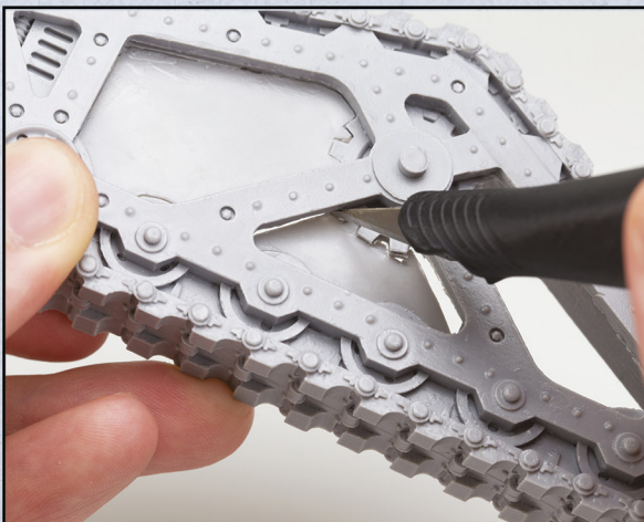
Shims are easily removed by cutting their edges with a modelling knife.
