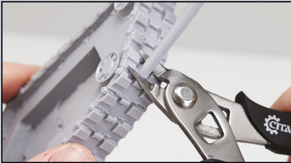
Clippers being used to remove the casting gates.
