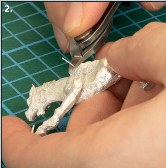
Clippers being used to remove stray metal vents.
